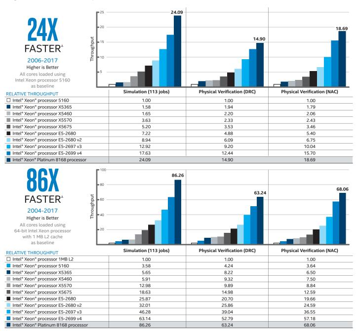
Figure 1. Electronic Design Automation (EDA) summary test results showing relative throughput of 64-bit Intel® Xeon® processors. Note: Same application binary used across all the platforms.
